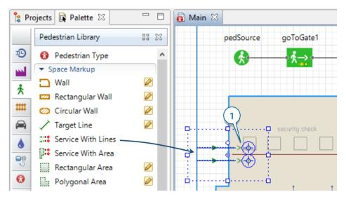
2. Open the **Service With Lines** properties area, use the **Name** box to name the shape *scpServices* - in this case, "scp" stands for security checkpoints - and then change the **Type of service** to *Linear*.
