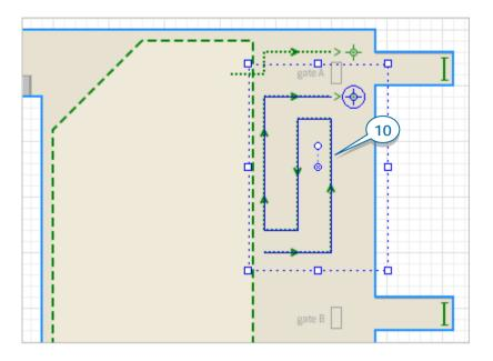
11. Draw an area at the gate with the **Rectangular Wall** element, and then add a table and two 3D woman models at the table. In the wall's properties, set **Visible** to **no** to make this wall invisible at the model runtime.
