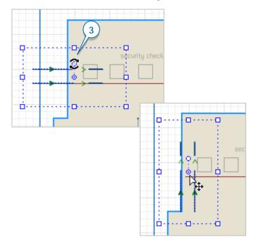
**4**. Move the service in a way that ensures the first linear service crosses the rectangle that represents the metal detector frame.
