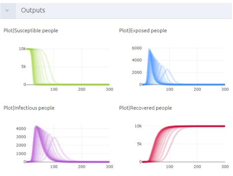
Each plot displays multiple curves (one for each simulation run) – 18 in total – in other words, 18 infection scenarios for contact rates that range from 0.3 to 2 – that represent the 18 steps in the parameter variation range that we defined earlier.
