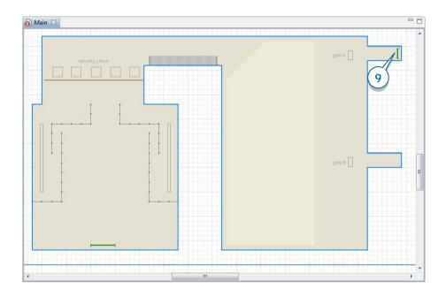
Your model's target line elements and space markup shapes must lie inside the walls. If any of your model's space markup shapes touch a wall, the "Exception during the discrete event execution: Unreachable target..." error message may display at the model runtime.
