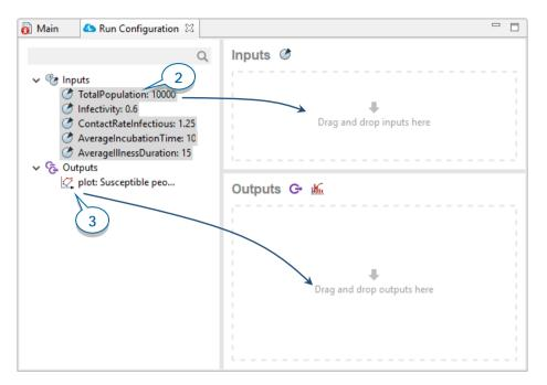
3. Do the same for the single output item (*plot*) – drag it from the **Outputs** tree branch to the **Outputs** section on the right.
