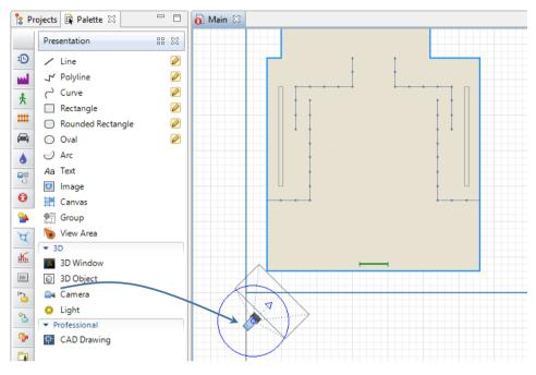
6. Drag the **3D Window** on to the *Main* diagram and place it below the terminal layout image.
