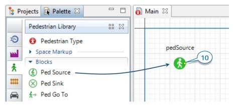
**11**. Since we want passengers to arrive randomly at an average rate of 100 passengers per hour, go to the *pedSource* block properties and then type *100* in the **Arrival rate** box.
