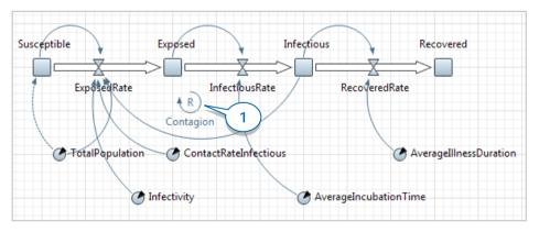
2. Go to the loop's **Properties**, change its **Type** to **R** (stands for Reinforcing), leave the default **Clockwise Direction**, and specify the text AnyLogic will display near the loop icon: *Contagion*.
