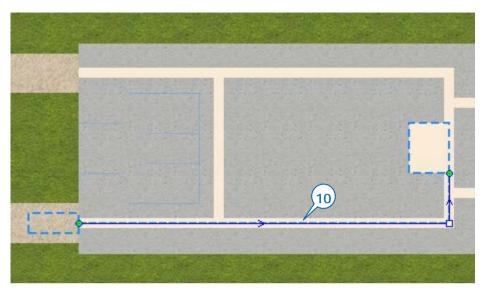
By default, paths in AnyLogic are bidirectional. However, you can limit movement along a selected path to one direction by clearing the **Bidirectional** property and then defining the movement direction. You can view a given path's direction by selecting the path and then viewing the direction arrow that displays in the graphical editor.
