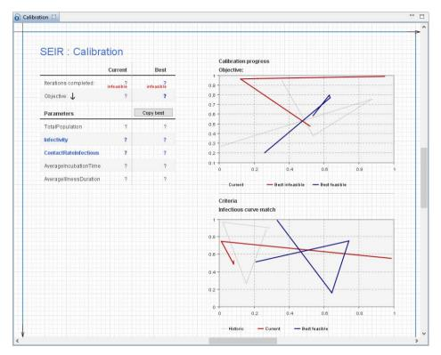
The image below shows the experiment's properties. Its objective is to minimize the difference between the model output and historical data.
