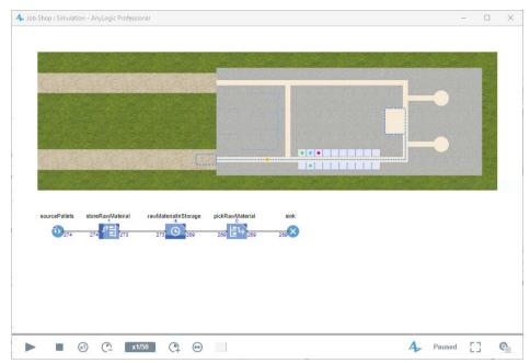
If the **Exception during discrete event execution** error message displays, you must connect your pallet rack to the network. You should select the pallet rack shape in the graphical editor, move it until the pallet rack's aisle displays a green highlight that shows it has connected to the network, and then rerun the model.
