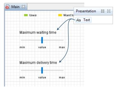
**16**. In the properties view, in the **Text** section, enter the text that the model will display. Using text shapes, name one slider *Maximum waiting time* and the other slider *Maximum delivery time*.
