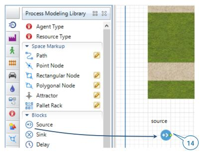
14. Drag the **Source** ⊕ element from the ⊕ **Process Modeling Library** palette on to the graphical diagram and name the block *sourcePallets*.
