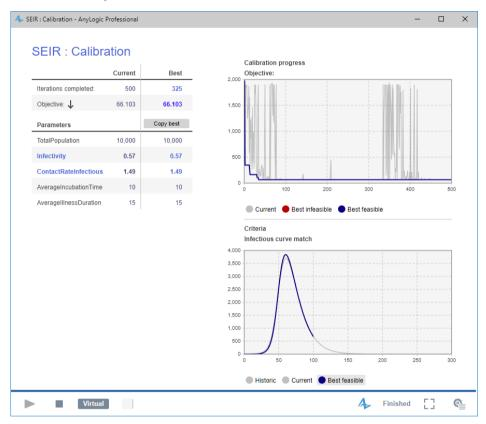
**13.** After the calibration is complete, you can copy the best fitting parameter values by clicking the **copy best** button in the model window and then paste them into the simulation experiment by clicking the **Paste from clipboard** button that you'll find on the *Simulation* experiment's properties page.
