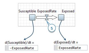
6. You can look at the formulas of *Susceptible* and *Exposed* stocks. Since our *ExposedRate* flow reduces the value of *Susceptible* stock and increases *Exposed*, the formulas should be the same as in the figures below. AnyLogic automatically created these formulas when you added the flow.
