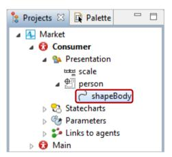
Here we call the function of *shapeBody*. To access the element's function, type the element name (*shapeBody*), type a dot, and then use the code completion feature to list the element's functions or select the function name from the list.
