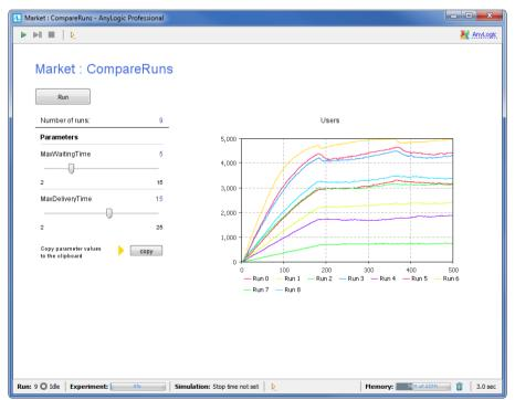
14. Each curve in a chart corresponds to a specific simulation run, and you can click any item in the chart's legend to highlight the curves that correspond to the run. The controls on the left will show the values that led to this result. To deselect a curve, click on its legend a second time.
