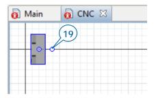
We're ready to use two similar 3D animation shapes to animate the CNC machine: one shape will represent the idle machine and the other will represent the machine as it processes the raw materials. We'll define dynamic values for each shape's **Visible** property that will allow our model to use the CNC machine's state to determine which shape the model will display at runtime.
