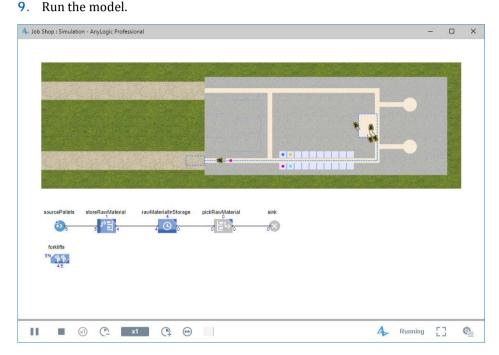
You'll see the forklift trucks pick up the pallets and store them in the pallet rack. After a brief delay, they move the pallets to the forklift truck parking area where the pallets will disappear.
