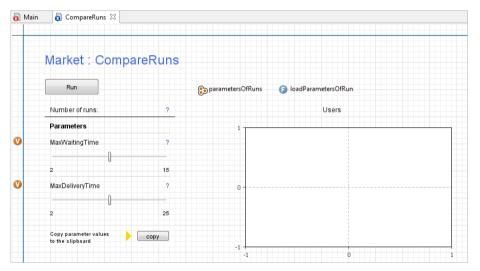
11. We want our experiment to simulate the model for just 500 days. To do this, select *CompareRuns* experiment in the **Projects** tree. In the experiment properties, open the **Model time** properties section, and type *500* in the **Stop time** field.
