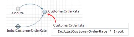
• An element is mentioned in the stock's initial value. This link type is drawn with a dotted line:
