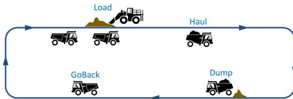
Figure 3-24: Cycle of earthmoving operation
