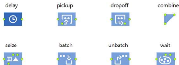
Figure 3-19: PML blocks that by default are set to pull protocol but can also support push
