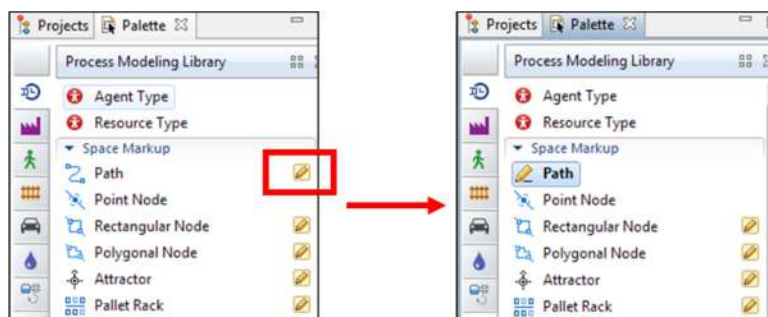
Figure 3-122: Double clicking the pencil icon takes the space markup element to drawing mode
