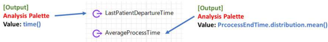
Figure 3-118: Output objects added to record the time of last patient departure and average processing time of 50 daily patients
